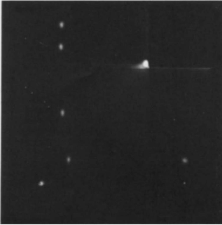
Fig. 5. Two-dimensional separation of milk extract contaminated with aflatoxin M 1 (0.1 µg/litre), prepared according to the method of Stubblefield (1979).
